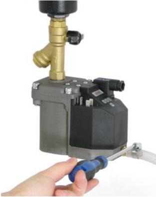
24. Replace the power cable, and optional alarm cable. Tighten the connector screw(s). **Max Torque 1Nm.** Make sure all gaskets are in place to ensure proper IP65 rating.
