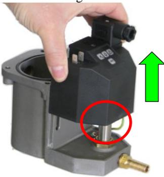
10. Unscrew the earth cable screw and place the electronics compartment aside where it will not get wet and/or damaged.
