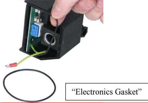
20. Slide the electronics compartment back on the housing bottom part and push it Down all the way.
