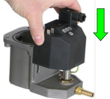
***WARNING: the electronics compartment is attached to the bottom housing part by cable (see Exploded View page 4). Do not damage this cable! Make sure it does get jammed!***
