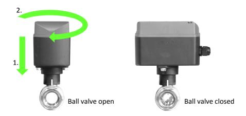
Please note: After a manual override the actuator will be 90° rotated versus the ball valve. All indicators and settings will become reversed, meaning the pre-programmed OPEN and CLOSE settings will become reverse, i.e. OPEN will become CLOSED and CLOSED will become OPEN.
