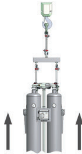
II: Installing by crane
