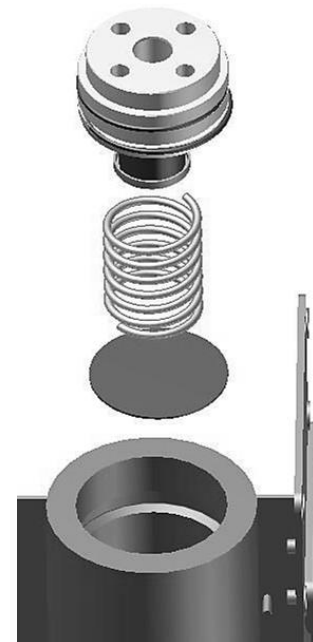
Piston, dust screen, spring and perforated plate
