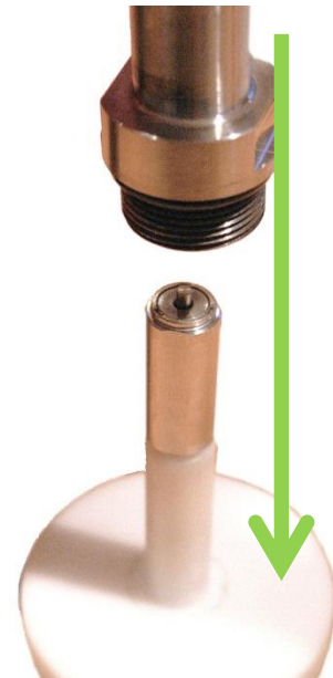
Valve armature gauge
