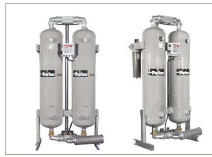
The K-MT 35-95 adsorption dryer series operates a fixed, timed, changeover-cycle between the two dryer vessels. Where the application calls for a unit able to cope with variations in operating pressure and load, the installation of a dew point sensor at the outlet of the dryer is available as an option: In such an operating mode, the changeover-cycle between vessels only takes place when required, and is
