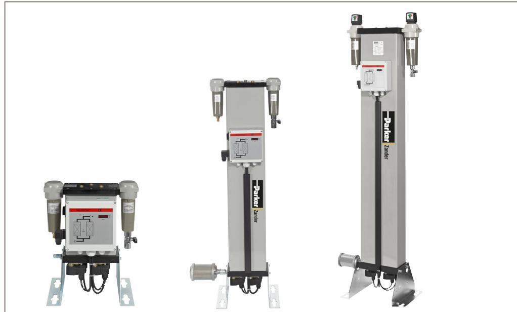
Dry compressed air finally exits via a validated GL after-filter preventing the migration of particles into the downstream compressed air network. The K-MT 1-8 adsorption dryer series operates a fixed, timed, changeover-cycle between the two dryer chambers. Where the application calls for a unit able to cope with variations in operating pressure and load, the installation of a dew point sensor at the outlet of the dryer is available as an option: In such an operating mode, the
