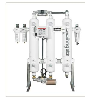
Dry compressed air subsequently enters the integral purification and catalytic stage where oil-vapour, odours, gaseous vapours and traces of carbon-monoxide are reliably removed. Finally, the clean, treated air exits via the validated GL after-filter into the downstream compressed air network.
