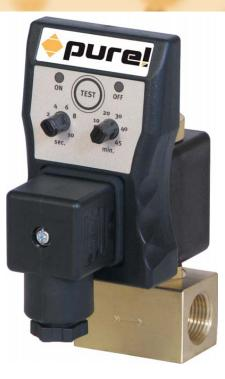
0.5 - 45 minutes, adjustable 0.5 - 10 seconds, adjustable 12 - 380 VAC/DC, 50/60 Hz 4mA maximum -40° C to +55° C IP 65, NEMA 4 when installed ABS plastic FR grade 43650ADIN ISO 4400 1 LED (yellow) indicating ON 1 LED (yellow) indicating OFF
