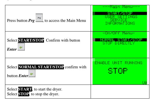
From the moment you select STOP in the controller, normally it passes quite a long time before the dryer really stops. In fact the dryer stops only when the regeneration cycle is completed. This to ensure a proper functioning of the system at the next restart.
