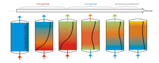
At the end of re generation time, the purge air is used to pressurize the column at the working pressure, the column is now ready for operation.
