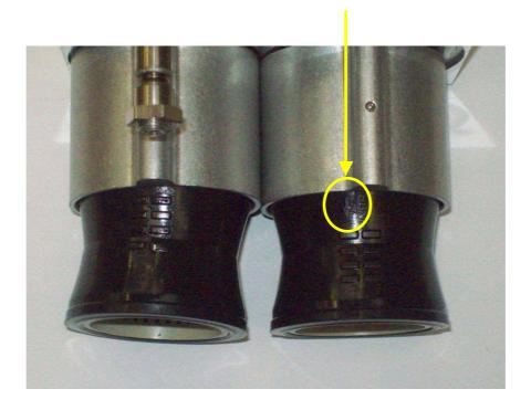
Arrow direction must be consistent with the direction of the air flowing through the valve.
