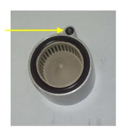
Arrows are marked on the valve rubber surface.
