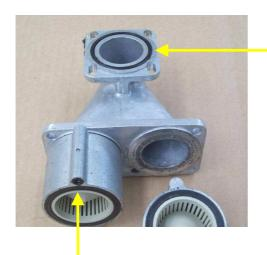
Replace the o-ring inserted between the flanges connecting tank with elbow.
