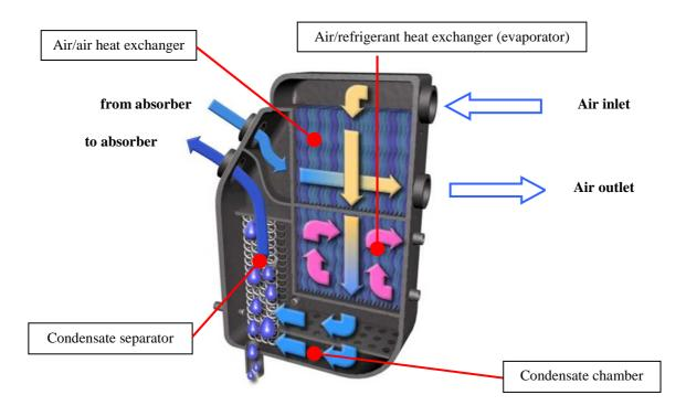
The water condensate produced inside the heat exchanger must be separated from the cold and dry air delivered to the desiccant columns.
