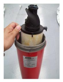
From the initial position (reference marks aligned), turn the filter body a couple of full turns to realign the ref. marks.
