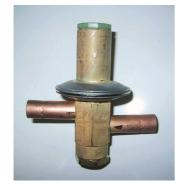
The cooling capacity regulation is made by means of the valve bypass hot gas: such valve by-passes part of the hot vapor refrigerant coming from the compressor, injecting it into the suction piping (evaporator outlet); thereby reducing the cooling capacity of the dryer if this exceeds the actual thermal load.
