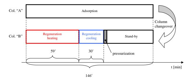
The electronic controller allows to set the dryer working pressure (parameter U2). Working times are automatically recalculated accordingly with pressure setting.
