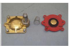
Remove the valve cover by loosening the fixing bolts.
