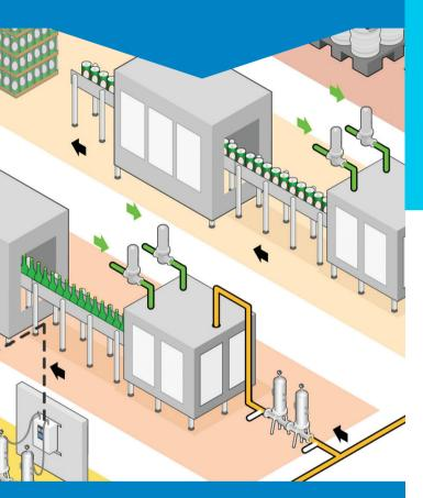
Cold stabilisation refers to the microfiltration of beer to remove any spoilage microorganisms before it is packaged.
