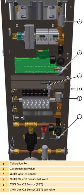
**Note**. The ball valves are shown in the normal operation position and should be returned to this position on completion of the calibration.
