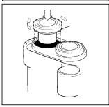
Remove existing pre-filter(s) & carbon bag(s) and dispose of in a responsible & legal manner.
