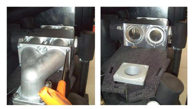
Replace the o-ring inserted between the flanges connecting tank with elbow.
