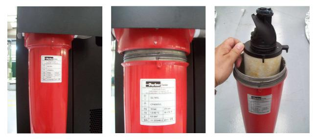
From the initial position (reference marks aligned), turn the filter body a couple of full turns to realign the ref. marks.
