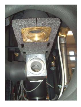
Replace the o-ring inserted between the flanges connecting tank with elbow.
