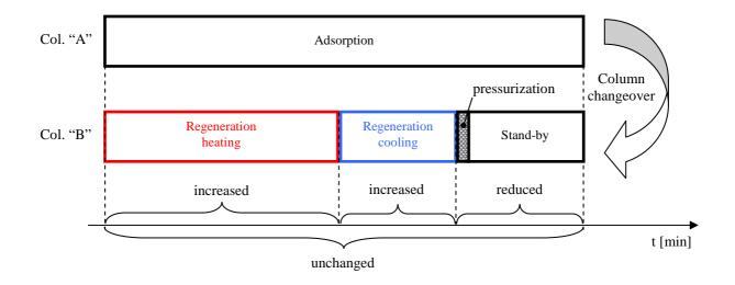
Working cycle with fixed time, setpoint  $\ge$  -40°C and pressure > 7 bar
