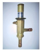
The cooling capacity regulation is made by means of the valve bypass hot gas: such valve by-passes part of the hot vapor refrigerant coming from the compressor, injecting it into the suction piping (evaporator outlet); thereby reducing the cooling capacity of the dryer if this exceeds the actual thermal load.. Pressure switches
