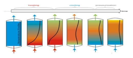
At the end of re generation time, the purge air is used to pressurize the column at the working pressure, the column is now ready for operation.
