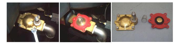
Remove the valve cover by loosening the fixing bolts.
