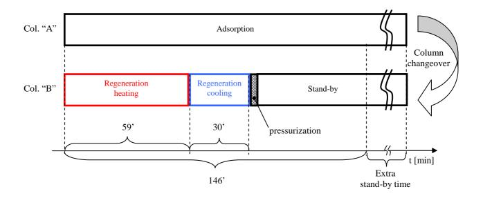
If a particularly deep drying is required (dewpoint lower than -40°C), the desiccant material must be regenerated more frequently. The electronic controller modifies the working cycle eliminating the time of stand-by.
