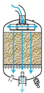
The regeneration phase starts with the column depressurization. In order to avoid sharp movements of the desiccant material inside the column, it is appropriate that the pressure is discharged from the lower side of the column.
