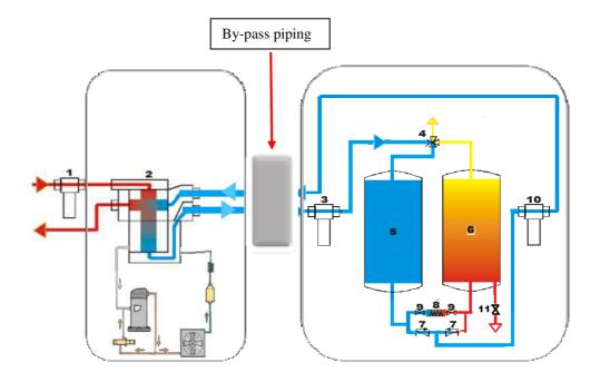
Il by- The by-pass is made by a pipe equipped with a solenoid valve (ATT140) or pneumatic valve (ATT260-340).
