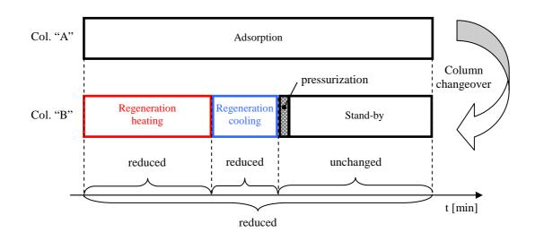
By setting parameter U6 = "fitted", the dewpoint control function is activated. Such function is available only if for dewpoint  $\geq -40^{\circ}$ C
