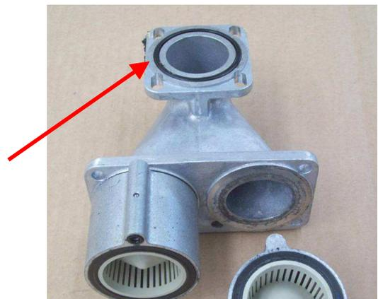
The side of aluminum casing equipped with o-ring must be positioned on the central part of the valve block.
