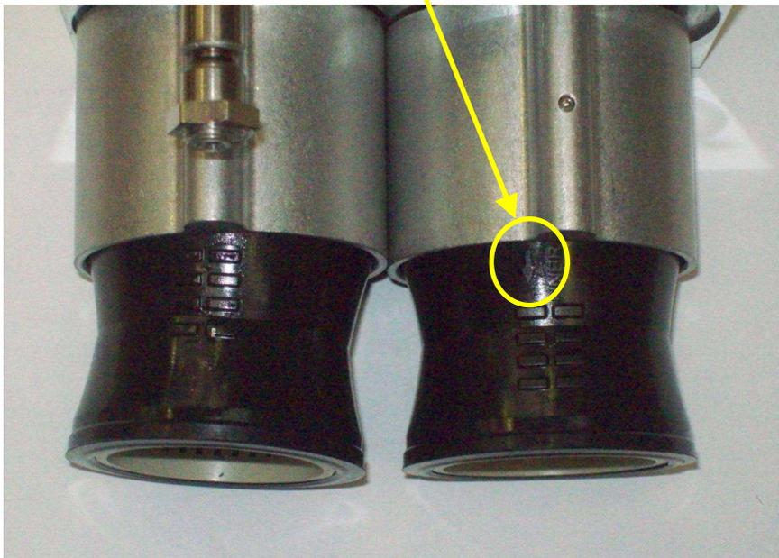
Arrow direction must be consistent with the direction of the air flowing through the valve.
