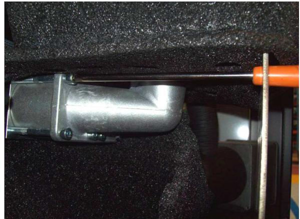
Replace the o-ring inserted between the flanges connecting tank with elbow.
