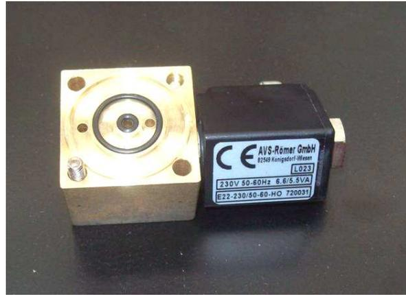
Remove the solenoid from the aluminum block valve by loosening the two fixing screws. Replace the damaged item or the whole piece in accordance with the program of periodic maintenance.
