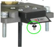
10. Unscrew the earth cable screw and place the electronics compartment aside where it will not get wet and/or damaged.
