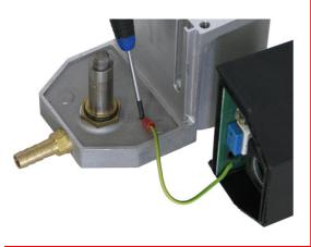
21. Replace the bottom part of the housing. Make sure the sensor does not get damaged!
