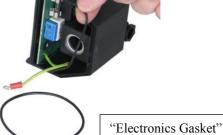
20. Slide the electronics compartment back
