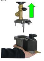
18. If needed, replace the *optionally available* electronics gasket under the electronics compartment by the electronics gasket supplied in the service kit. *Use a lubricant for proper sealing*.
