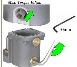
17. If needed, replace the <u>optionally available</u> large housing O-ring with the one supplied in the service kit. *Use a lubricant for* proper sealing.
