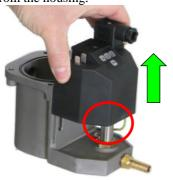
WARNING: the electronics compartment is attached to the bottom housing part by a cable (see Exploded View page 4). Do not damage this cable!
