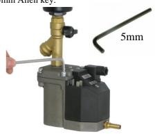
8. If needed, replace the *optionally available* small O-Ring on the sensor module. *Use a* lubricant for proper sealing.
