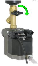
2. Press the TEST button to empty the unit of any residual condensate and to depressurise the KAPTIV-CS.
