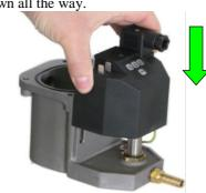
WARNING: the electronics compartment is attached to the bottom housing part by cable (see Exploded View page 4). Do not damage this cable! Make sure it does get jammed!
