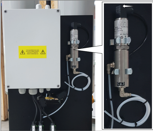
(a) Back panel and Michell hygrometer assembly
