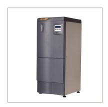
The Parker domnick hunter zero nitrogen generators employ robust, field proven technology to produce ultra high purity nitrogen for GC makeup and carrier gas applications. An integral heated platinum catalyst ensures carrier grade nitrogen free from organic impurities to <0.1ppm.
