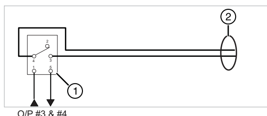
Fault Relay Configuration
