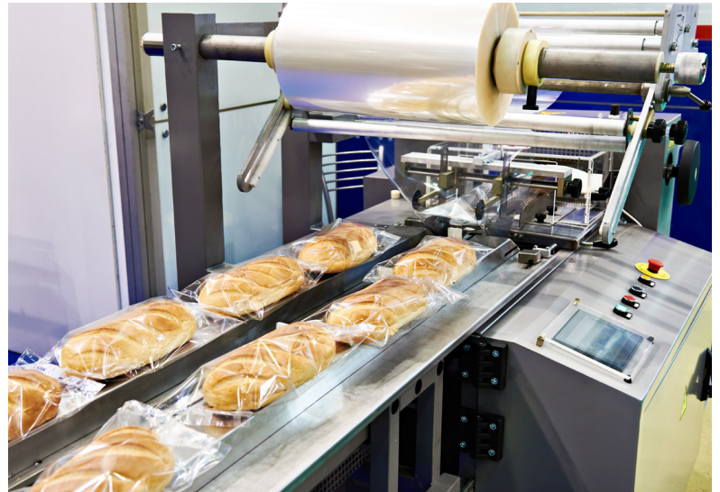
HFFS, (Flow wrapper packaging bakery products).
